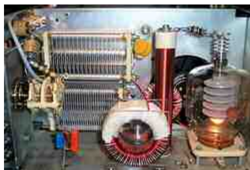
Eric Tichansky, NO3M, has modified a Heathkit SB-1000 linear for 630 meters, so he can generate sufficient power to obtain 1 W ERP.
